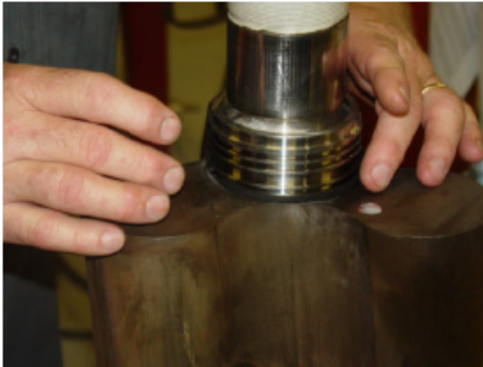
FIGURE 7-1 – INSTALL PISTON RINGS
