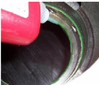
FIGURE 7-3 – LOCTITE 620 BEARING HOUSING
