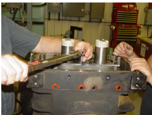
FIGURE 7-10 – TORQUE THE SCREWS 38-41 FT. LBS.
