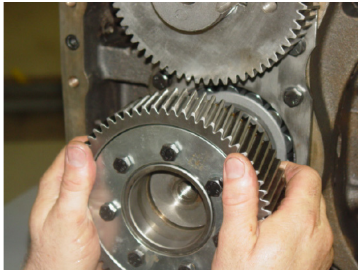
FIGURE 7-13 – HOLDING GEAR ASSEMBLY TOGETHER SLIDE ON SHAFT
