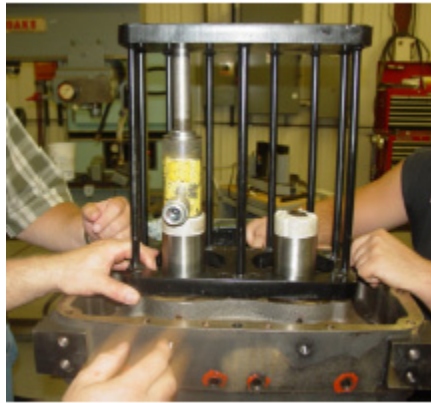
FIGURE 6-1 – CYLINDER SET UP ON BOTH SHAFTS
