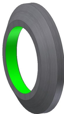
Figure 7-7 – LOCTITE 620 APPLIED TO INTERNAL SLINGER
