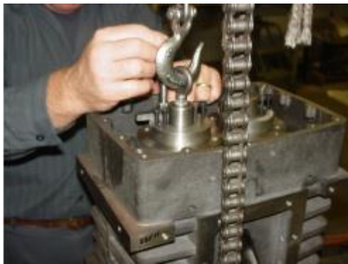
FIGURE 8-2 – MEASURE STEP IN FALSE BEARING
