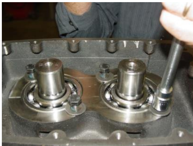
FIGURE 8-4 – INSTALL BEARING RETAINING SCREWS
