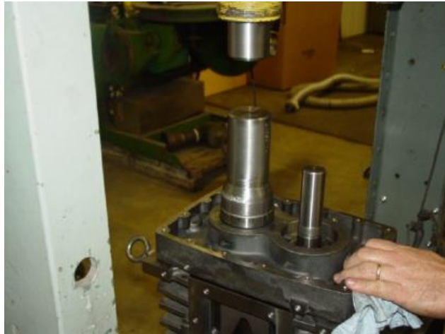
FIGURE 8-3 – PRESS BEARING ONTO ROTOR SHAFT
