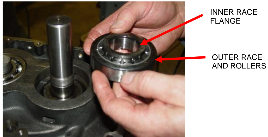
FIGURE 8-5 – INSTALL ROLLER BEARING
