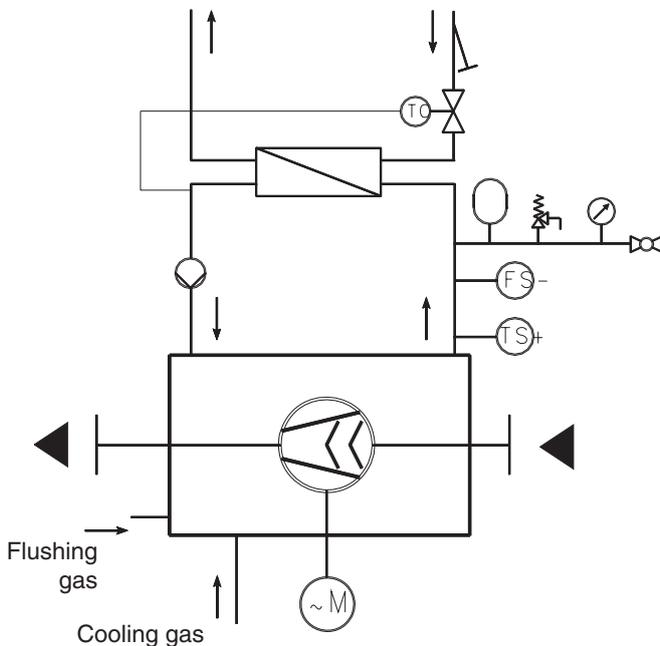
**Water-water radiator:** The external cooling circuit is connected to the factory's main water supply. It is equipped with a dust trap and a temperature controlled valve. This valve remains closed during the start run of the pump.
