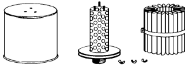
FIGURE 4-6 – DRY TYPE FILTER AND FILTER-SILENCER
