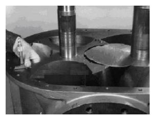
FIGURE 7-9 – DEPTH MICROMETER
