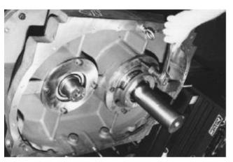
FIGURE 6-8 – BEARING CLAMP PLATE
