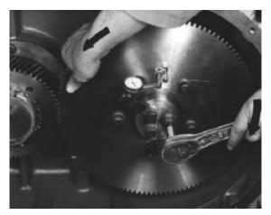
FIGURE 7-29 – SETTING THE INTERLOBE CLEARANCE
