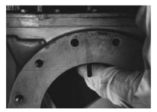
FIGURE 7-18 – DISCHARGE END CLEARANCE CHECK
