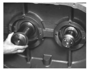
FIGURE 7-24 - SLIDE SHIMS OVER SHAFT ASSEMBLY
