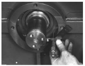
FIGURE 7-21 – BEARING BORE
