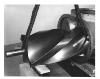
FIGURE 6-10 - ROTOR REMOVAL
