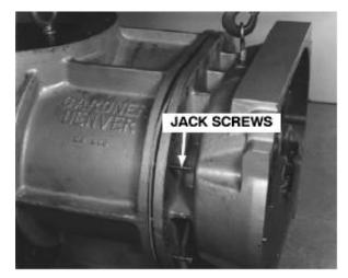
FIGURE 6-11 – BEARING CARRIER
