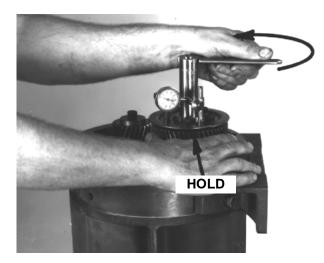
**Example**: if the indicator reading in Step 19 is +15, then move the rotor clockwise until the indicator reads +10. Tighten the gear to hub Nylok type screws evenly. Be sure the indicator reading does not change. The rotors are held in time by the clamping action of the screws and distortion of flat washers into slotted holes in the gear. Rotate rotors to be sure timing has not slipped and there
