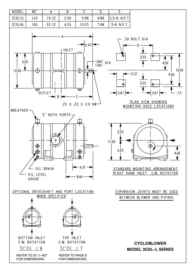
FIGURE 4 - OUTLINE DIMENSIONS - RIGHT HAND INLET (STANDARD)
