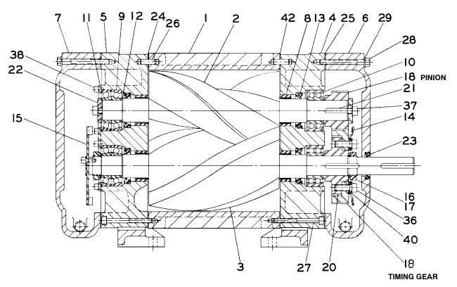
NOTE: This drawing covers Right Hand Air Inlet, Bottom Air Inlet and Top Air Inlet Arrangements. For Top and Bottom Air Inlet, Oil Level Gauge must be relocated in the highest hole in the End Cover.
