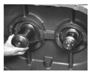
FIGURE 7-24 - SLIDE SHIMS OVER SHAFT ASSEMBLY
