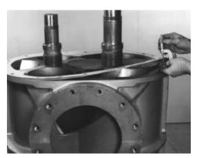
FIGURE 7-10 - OUTSIDE MICROMETER
