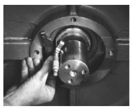
FIGURE 7-22 - DEPTH MICROMETER
