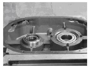
**FIGURE 7-6 – BEARING INSTALLATION**
