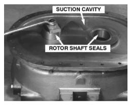
FIGURE 7-1 - ROTOR SHAFT SEAL
