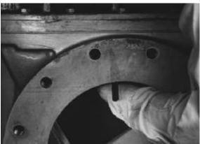
FIGURE 7-18 . DISCHARGE END CLEARANCE CHECK
