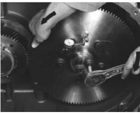
FIGURE 7-27 - SMALLEST MINUS READING
