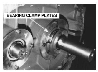
FIGURE 7-17 - BEARING CLAMP PLATES
