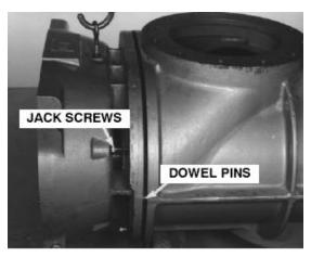
FIGURE 6-7 - BEARING CARRIER
