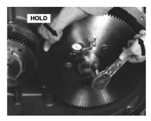
FIGURE 7-30 – HOLD GEAR & SHAFT FROM TURNING TIGHTEN FIVE GEARS TO HUB
