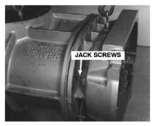
FIGURE 6-11 - BEARING CARRIER
