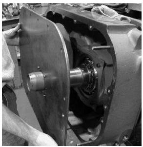
FIGURE 7-20 - END COVER ASSEMBLY
