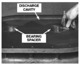
FIGURE 7-7 – DISCHARGE END BEARING CARRIER 37-1-616 Page 45
