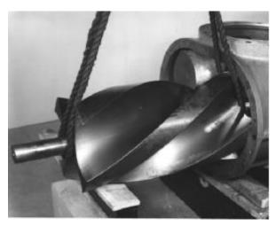
FIGURE 6-10 - ROTOR REMOVAL
