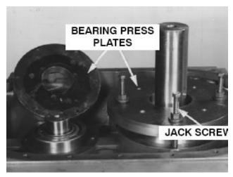
FIGURE 7-16 - BEARING PRESS PLATE
