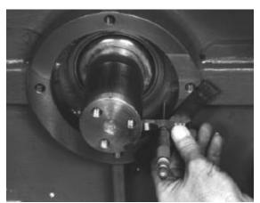
FIGURE 7-21 - BEARING BORE
