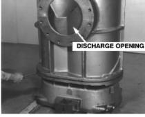
FIGURE 7-3 - DISCHARGE OPENING
