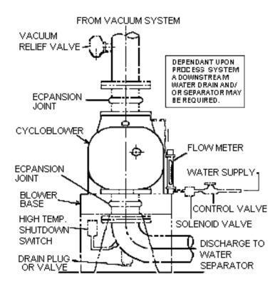
FIGURE 3-2- INLET WATER INJECTION DIAGRAM
