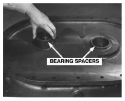
FIGURE 7-2 - BEARING SPACER
