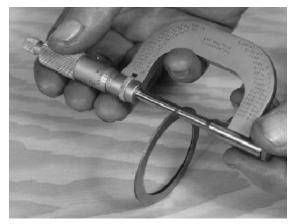
FIGURE 7-14 - BEARING SHIMS
