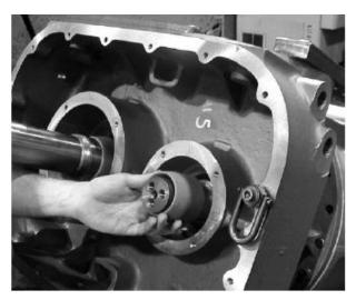
FIGURE 7-13 – SEAL INSTALLATION GUIDE
