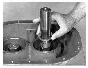
FIGURE 7-15 - BEARING SHIMS
