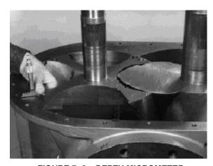
FIGURE 7-9 - DEPTH MICROMETER
