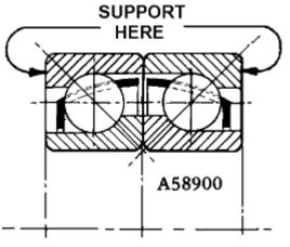
FIGURE 7-5 – ANGULAR CONTACT BEARING ASSEMBLY
