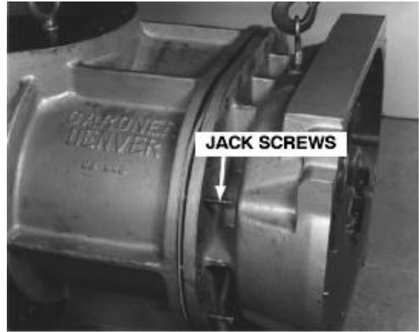
**FIGURE 6-11 – BEARING CARRIER**
