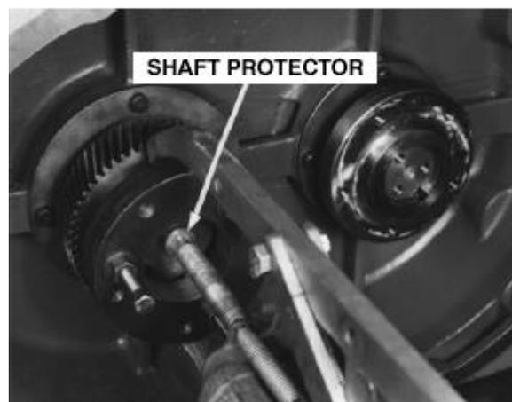
FIGURE 6-4 – BEARING PRESS PLATE
