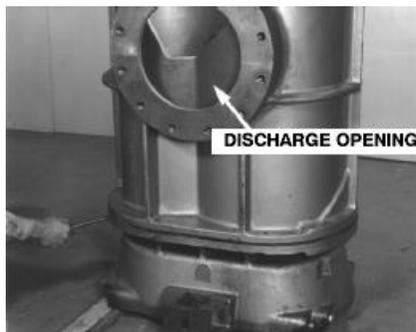
**FIGURE 7-3 – DISCHARGE OPENING**
