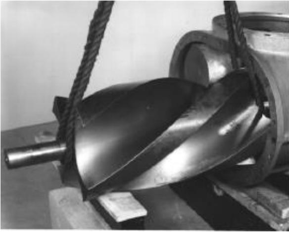
**FIGURE 6-10 – ROTOR REMOVAL**
