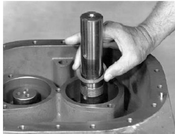
**FIGURE 7-15 – BEARING SHIMS**
