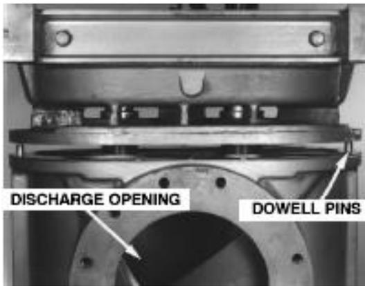
FIGURE 7-11 – DISCHARGE OPENING
