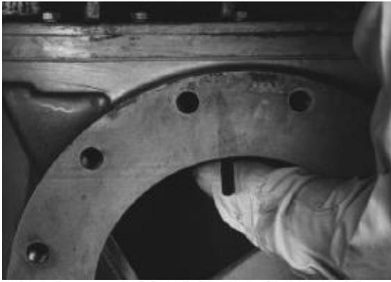
FIGURE 7-18 . DISCHARGE END CLEARANCE CHECK
