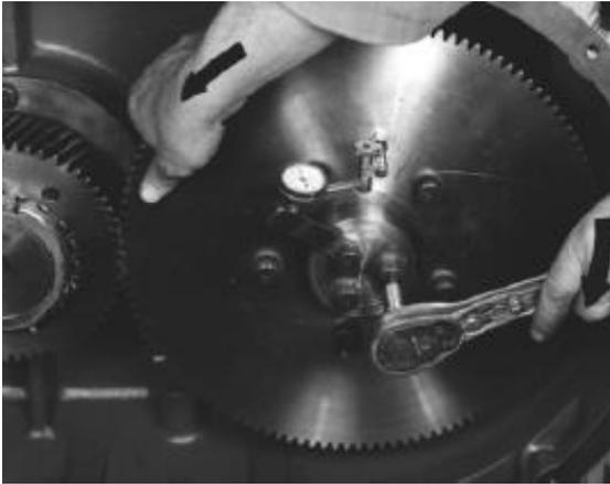
**FIGURE 7-29 – SETTING THE INTERLOBE CLEARANCE**
