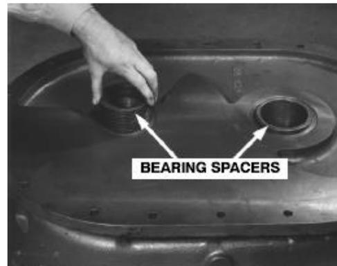
**FIGURE 7-2 – BEARING SPACER**
