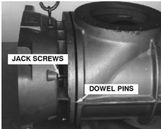
**FIGURE 6-7 – BEARING CARRIER**
