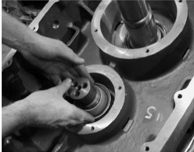
**FIGURE 7-23 – OIL SEAL ON GATE ROTOR SHAFT ASSEMBLY**
