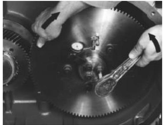
**FIGURE 7-28 – SMALLEST PLUS READING**
