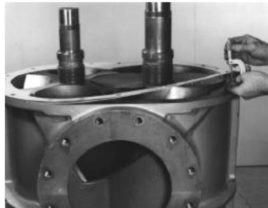
**FIGURE 7-10 – OUTSIDE MICROMETER**
