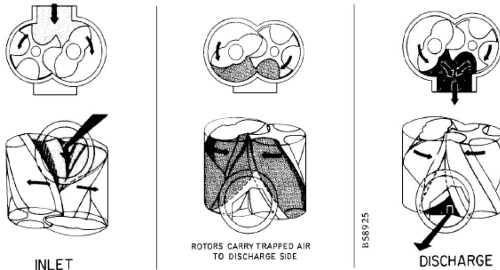
**FIGURE 2-1 – OPERATING PRINCIPLE**
