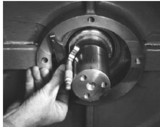
**FIGURE 7-22 – DEPTH MICROMETER**
